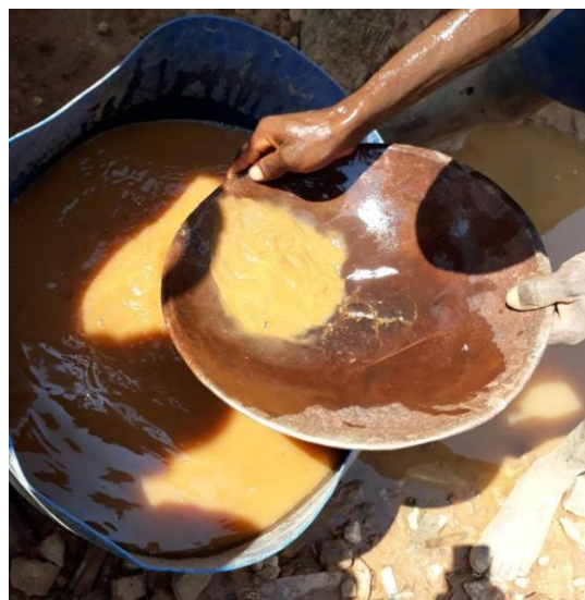
A miner mixing the concentrated gold ore with water and mercury to make an amalgam
